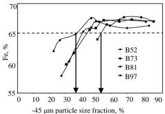
Fig. 5. Davis tube separation results of Dönentaş formation according to the content of the -45  $\mu$ m particle size fraction in the feed sample
