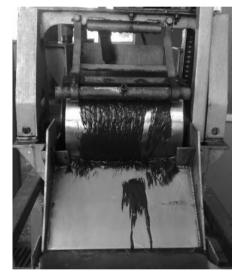
Fig. 2. Laboratory size low intensity drum type wet magnetic separator
