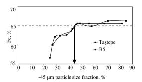
Fig. 4. Davis tube separation results of Taştepe formation according to the content of the -45 μm particle size fraction in the feed sample
