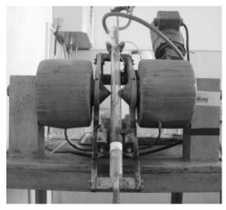
Fig. 1. Laboratory Davis tube magnetic separator
